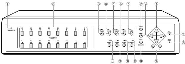
This unit is not equipped with a power switch. The power is turned on/off when the supplied power cord is connected/disconnected at the power source.
